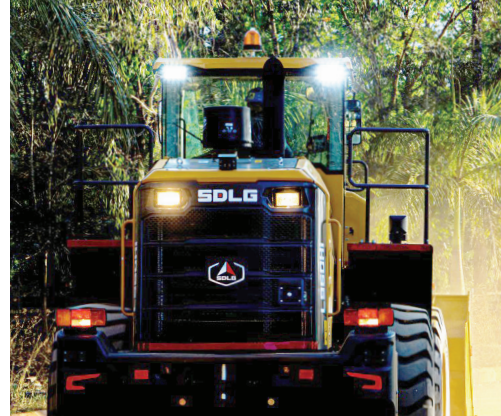
LED & Extra Working lights, reverse horn, and rotating beacon for better visibility
