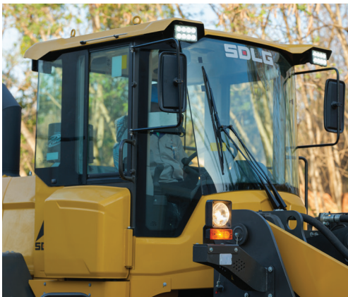
Features a spacious pressurized and shock-absorbing ROPS / FOPS Certified cabin with clear visibility, low noise, minimal vibration, and fast cooling air conditioning for a better working experience.
